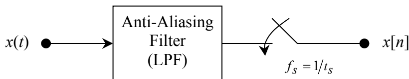
Figure 1: Continuous Time to Discrete-Time Conversion
