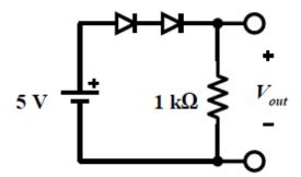
• Construct the circuit below, what is the output voltage now? Vary the supply voltage by  $\pm 2V$  and record the changes at the output voltage.
