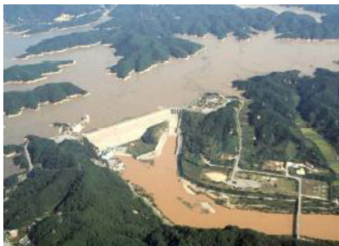
Fig. 1. Intrusion of highly turbid waters into Imha Reservoir during Typhoon Maemi in 2003 (reprinted with permission from the Korea water resources corporation)
