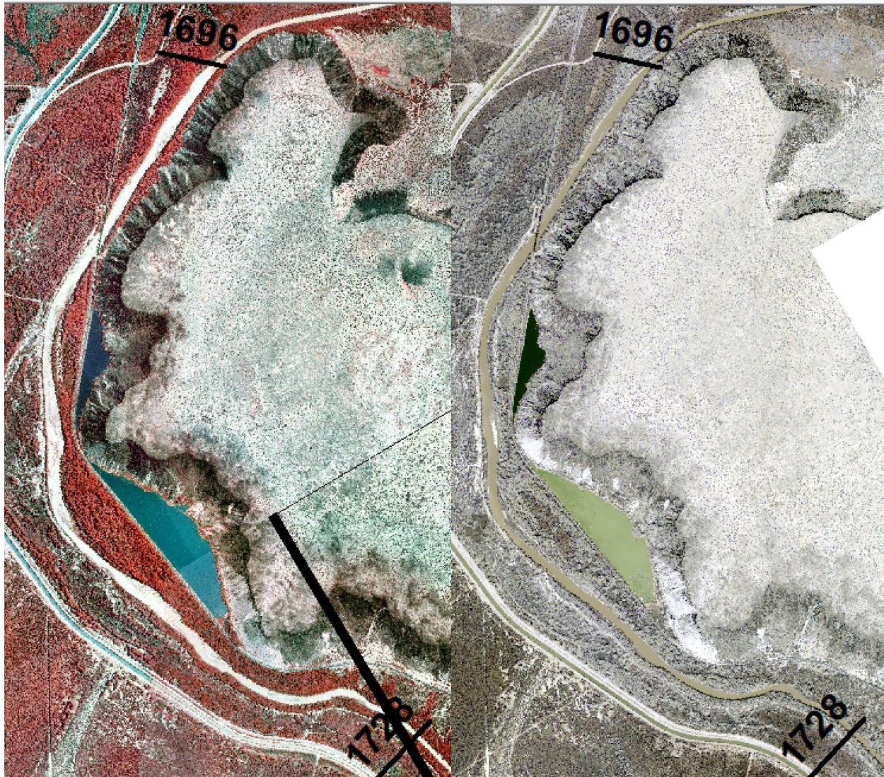
Figure 47 Aerial Photograph of subreach EB3 when multiple alternating bars, point bars, and islands were present in 2002 (left) and in 2012 (right) after vegetation encroachment.
