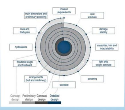
Iterative design. Maturation of the design proceeds from the outer ring to the inner through four main phases of development
