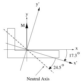
Step 7: Determine Maximum Tensile and Compressive Stress
