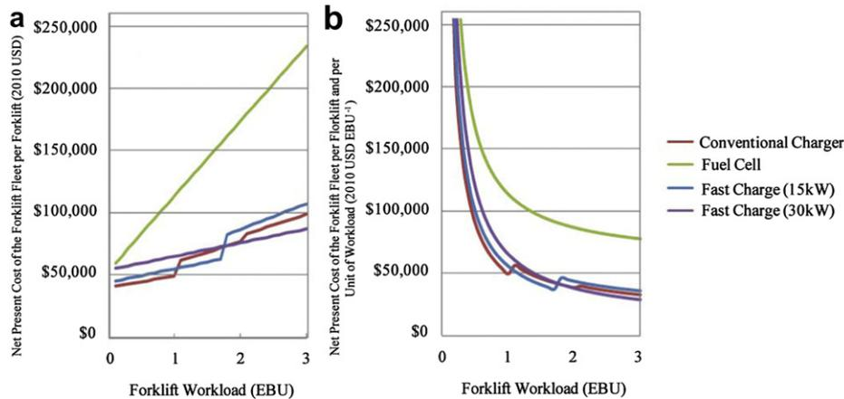
**Fig. 2 – Comparison of project net present cost (NPC) among the technologies modeled for two metrics of comparison: NPC per forklift, and NPC per forklift per unit of workload, measured in equivalent battery units (EBU).**
