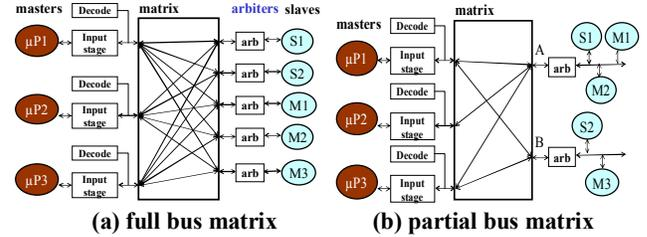
Fig. 2 Bus matrix architecture
