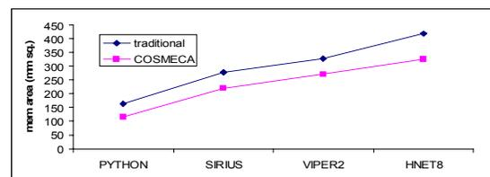
Fig. 10 Comparison of best solution memory area
