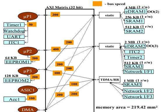
**Fig. 7 Synthesized output for SIRIUS**
