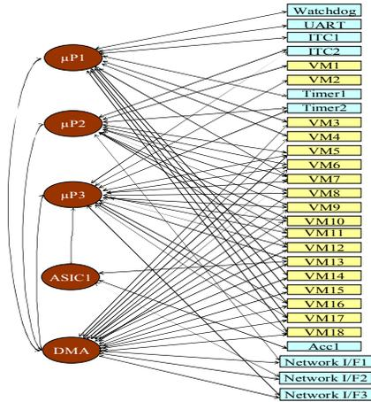
**Fig. 6 SIRIUS Communication Throughput Graph (CTG)**
