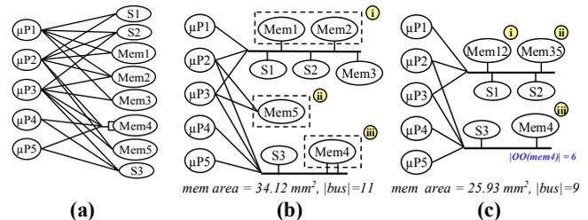
Fig. 1 (a) MPSoC system example with (b) memory synthesis before communication architecture synthesis, and (c) co-synthesis of memory and communication architectures
