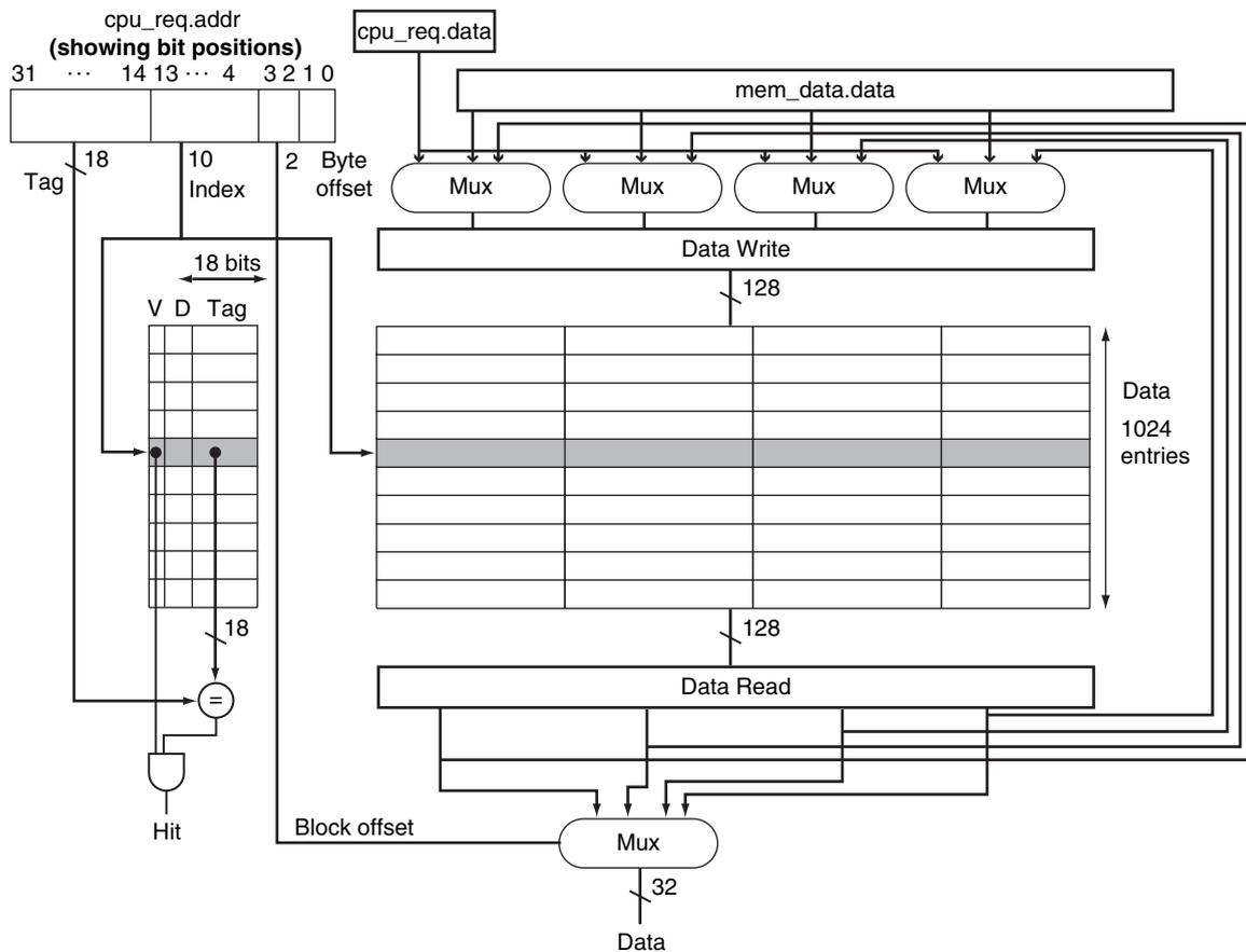
**FIGURE 5.9.3** Block diagram of the simple cache using the Verilog names. Not shown are the write enables for the cache tag memory and for the cache data memory, or the control signals for multiplexors that supply data for the Data Write variable. Rather than have separate write enables on every word of the cache data block, the Verilog reads the old value of the block into Data Write and then updates the word in that variable on a write. It then writes the whole 128-bit block.
