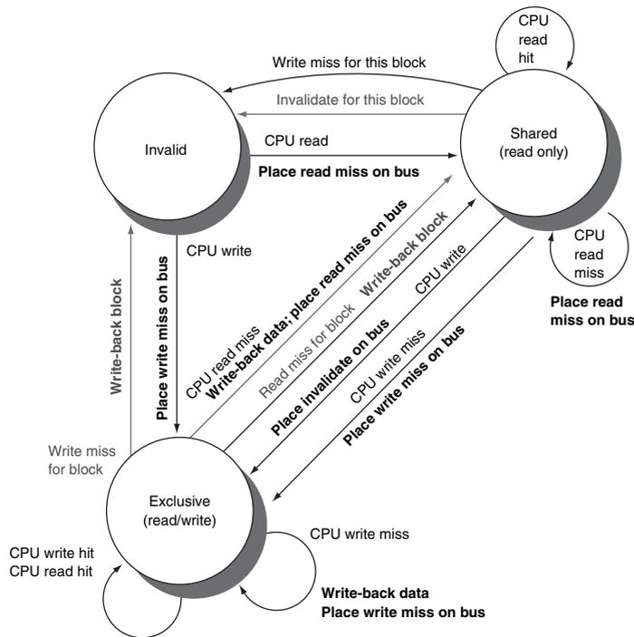
**FIGURE 5.9.11** Cache coherence state diagram with the state transitions induced by the local processor shown in black and by the bus activities shown in gray. As in Figure 5.9.10, the activities on a transition are shown in bold.
