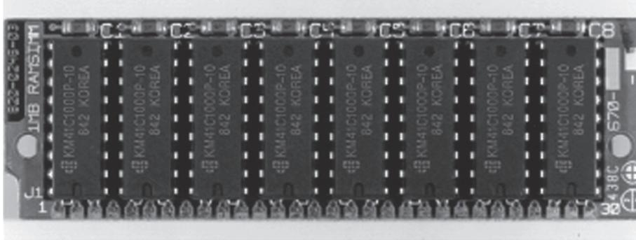
**FIGURE 5.13.4 A 1 MB SIMM, built in 1986, using 1 Mbit chips.** This SIMM sold for about \$5/MB in 1997. As of 2006, most main memory is packed in DIMMs similar to this, though using much higher-density memory chips (1 Gbit).
