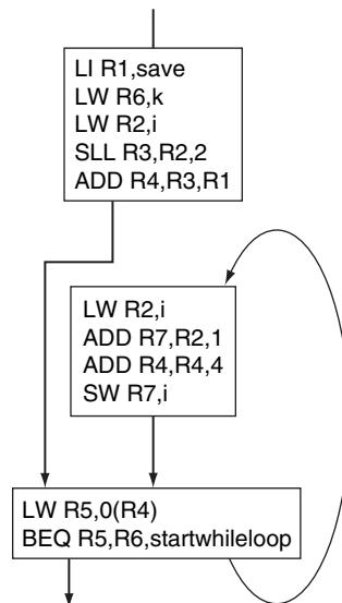
**FIGURE 2.15.5** The control flow graph showing the representation of the *while* loop example after code motion and induction variable elimination. The number of instructions in the inner loop has been reduced from 10 to 6.
