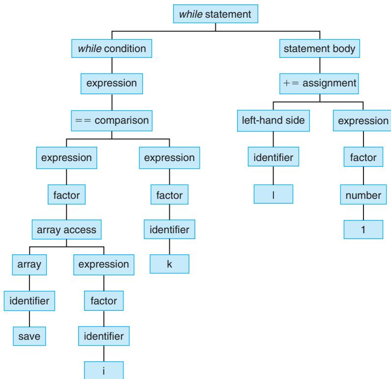
**FIGURE 2.15.2 An abstract syntax tree for the `while` example.** The roots of the tree consist of the informational tokens such as numbers and names. Long chains of straight-line descendants are often omitted in constructing the tree.
