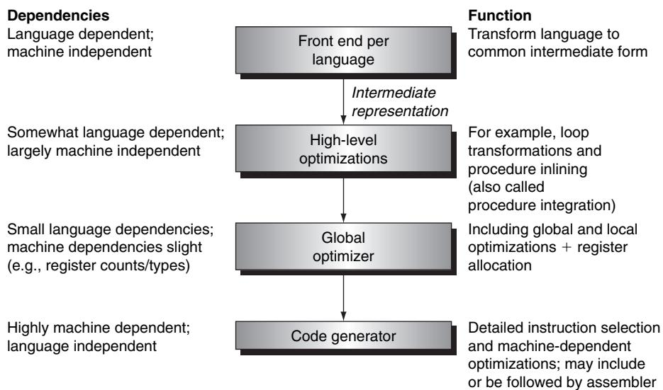
**FIGURE 2.15.1** The structure of a modern optimizing compiler consists of a number of **passes or phases**. Logically, each pass can be thought of as running to completion before the next occurs. In practice, some passes may handle a procedure at a time, essentially interleaving with another pass.
