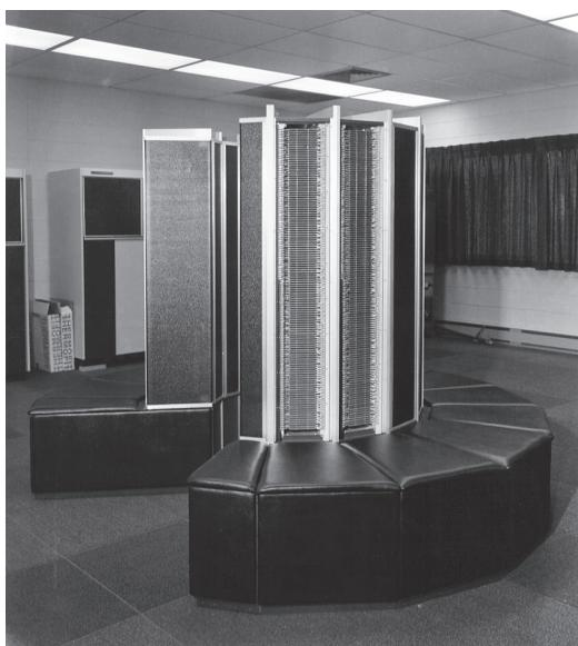
**FIGURE 1.10.4 Cray-1, the first commercial vector supercomputer, announced in 1976.**
