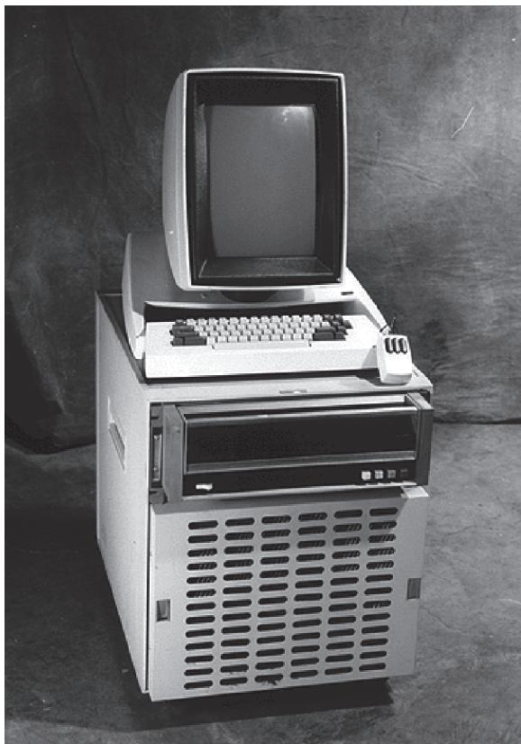
**FIGURE 1.10.6 The Xerox Alto was the primary inspiration for the modern desktop computer.** It included a mouse, a bit-mapped scheme, a windows-based user interface, and a local network connection.
