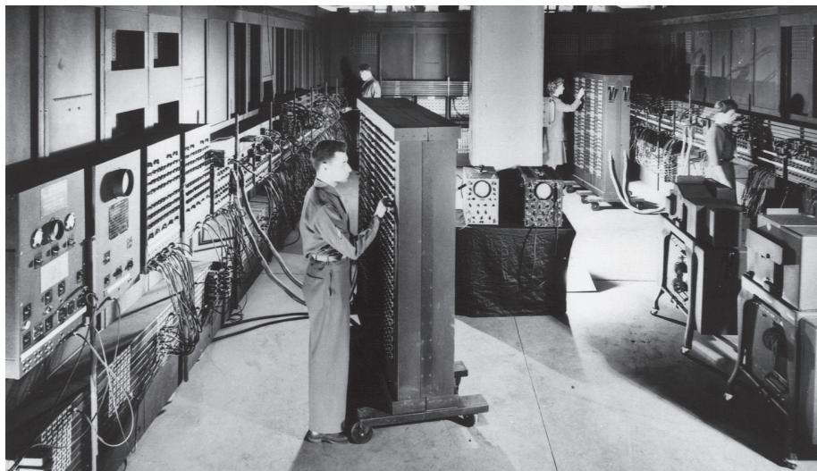
**FIGURE 1.10.1** ENIAC, the world’s first general-purpose electronic computer.
