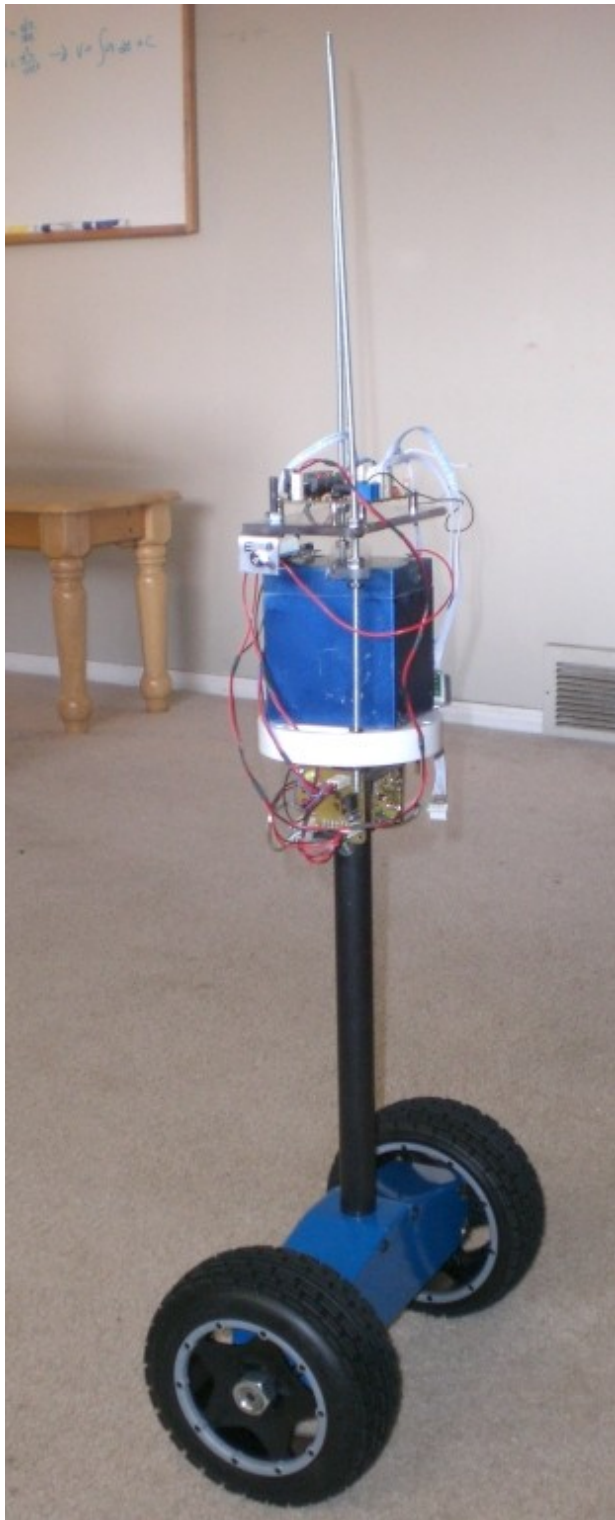
Picture 4: This is the demo system balancing in my living room. The enclosure for the electronics is not yet complete. The rods on top are just temporary mounting rods that have not been cut yet.
