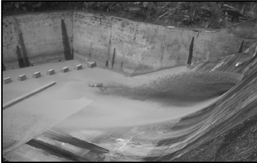
Figure 11: Thick Concentrated Sludge Gushing out from Hollow Jet Valve at 2 in (5.1 cm) Opening.
