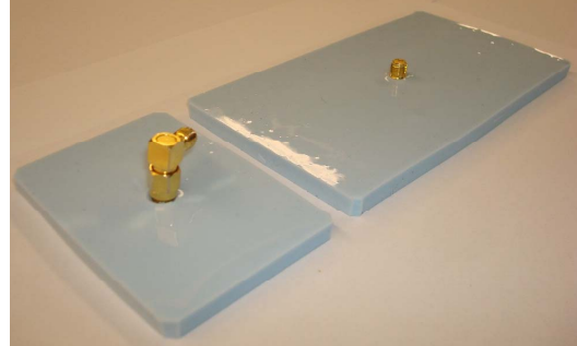
Fig. 5. Silicone molded antenna. The antennas molded are of the same type as shown on Fig.1. The mold in the front contains a 2.45 GHz and a 1.575 MHz antenna, combined size 55mm x 80mm. The bigger mold in the back contains a 915 MHz and a 1.575 MHz antenna of the same type, combined size 80 mm x 125 mm. The antennas are perpendicular to each other and parallel to the sides of the mold. The thickness of the mold is 6mm. The antenna plane is in the center of the mold.
