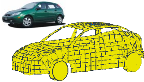
Fig.1. MoM-PO model of an automobile with an oblique monopole rooftop antenna.
