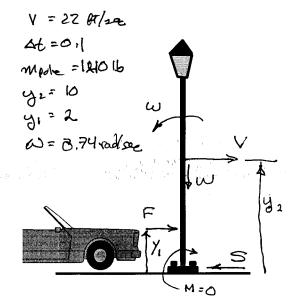
a. From the principle of linear impulse and momentum write an equation including the shear force S.
