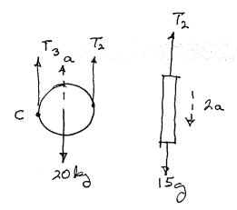
b. Calculate the upward acceleration,  $a_0$  of the disk center 0 and the cable tension, T, between disk and counterweight.
