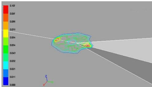
Figure 5: Hypothetical Porton Trial No. 8 spill surface concentrations with gorge slope 1:10, sidewall slope 1:4.14 at t = 40 sec.
