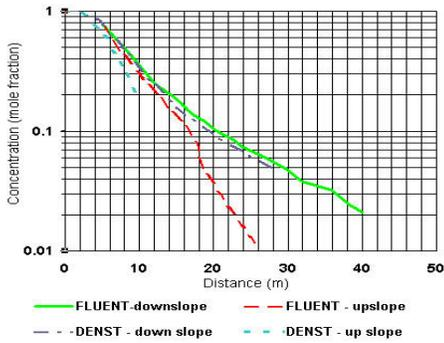
Figure 3: Hypothetical Porton Trial No. 8 spill on 1:20 slope, concentrations vs. distance.
