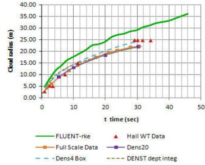
Figure 2: Porton Trial No. 8, gas cloud radius vs. time.
