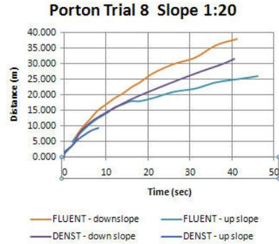
Figure 4: Hypothetical Porton Trial No. 8 spill on 1:20 slope, cloud radius vs time.
