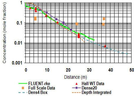
Figure 1: Porton Trial No. 8, gas cloud peak concentrations vs. distance.
