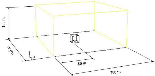
Figure 2. Schematic 3-d generic building atrium, symmetric door openings.
