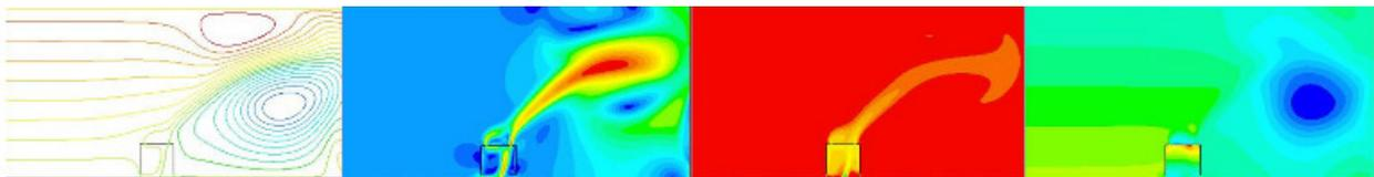
Figure 8. Stream lines, velocity magnitude, density and static pressure contours, 2-d Building, Up and downwind door openings,  $U = 1$  m/s,  $t = 35$  sec.
