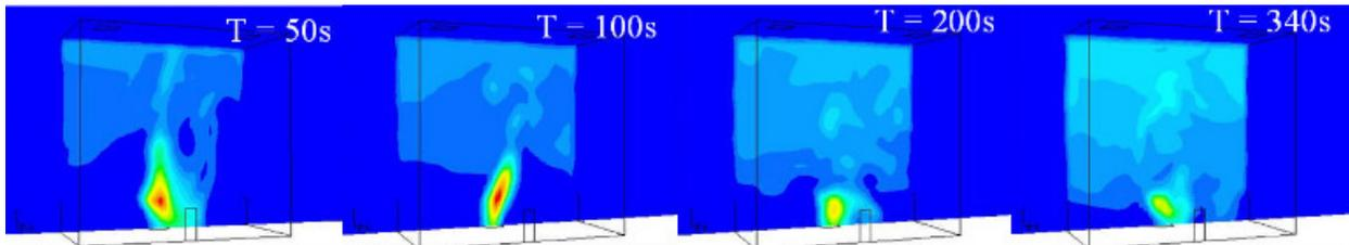
Figure 11. Temperature Contours 3-d Building,  $U = 2$  m/sec.  $t = 50, 100, 200$  and  $340$  sec. Symmetric door openings.
