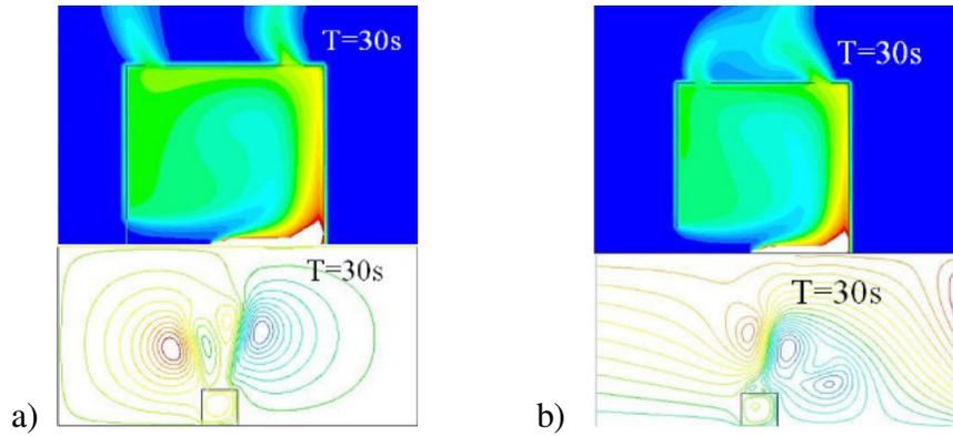
Figure 9. 2-d Building, Upwind door openings, Temperature contours and Stream lines,  $t = 30$  sec.
