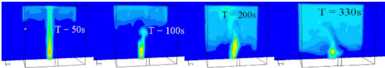
Figure 10. Temperature Contours 3-d Building,  $U = 0$  m/sec.  $t = 50, 100, 200$  and  $330$  sec. Symmetric door openings.
