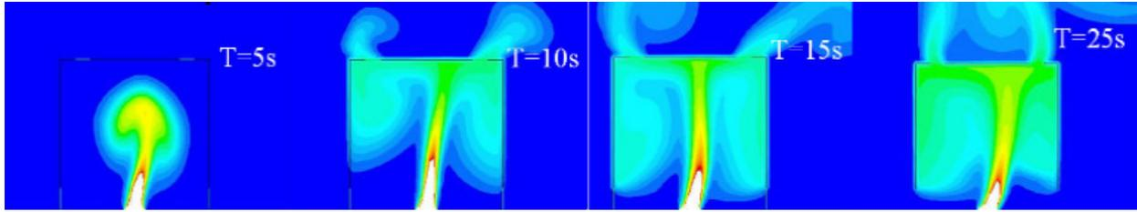
Figure 5. Temperature Contours 2-d Building, Up and downwind door openings,  $U = 0.5$  m/s,  $t = 5, 10, 15,$  and  $25$  sec.
