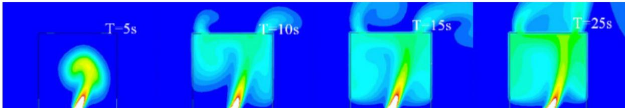
Figure 7. Temperature Contours 2-d Building, Up and downwind door openings,  $U = 1$  m/s,  $t = 5, 10, 15,$  and  $25$  sec.
