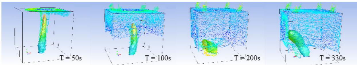
Figure 12. Temperature Contours 3-d Building,  $U = 2$  m/sec.  $t = 50, 100, 200$  and  $330$  sec. Asymmetric door openings.
