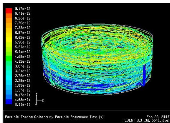
Pathlines of sludge recirculated through external mixer
