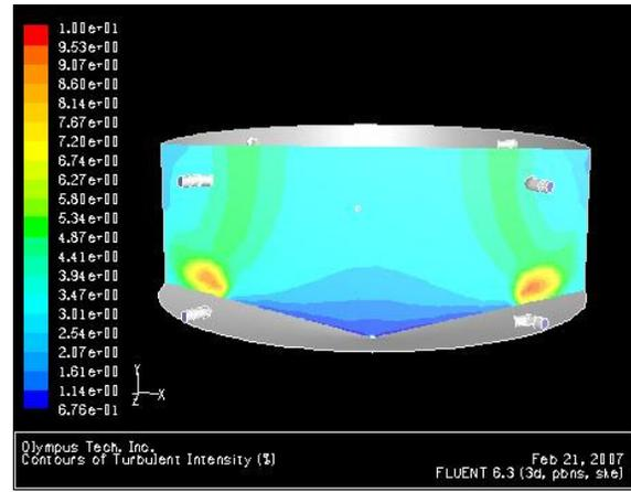
Turbulence intensity (mixing)
