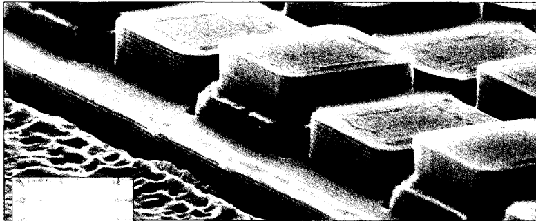
In this scanning electron micrograph, the "checkerboard" is in actuality a two-dimensional phased-locked array of vertical-cavity surface-emitting lasers. Molecular beam epitaxy was employed to grow the semiconductor wafer, complete with mirrors [light and dark stripes], and the result was topped by a thick phase-shift layer [solid light layer]. Then reactive ion beam etching was used to define each laser individually as a square, measuring 5 \mu\text{m} on a side, and the thick phase-shift layer was etched off the top of every other laser in the array. The inset is an optical micrograph of light emitted from the operating array.
