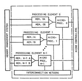
Figure 1. Block Diagram Overview of PASM.
