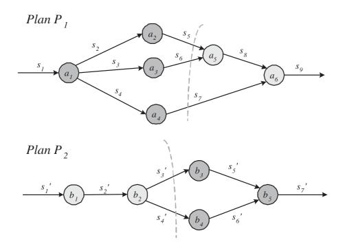
Figure 4. An example of execution switching between two plans. Snapshot  $[s_3', s_4']$  in Plan  $P_2$  is congruent to snapshot  $[s_5, s_6, s_7]$  in Plan  $P_1$ .
