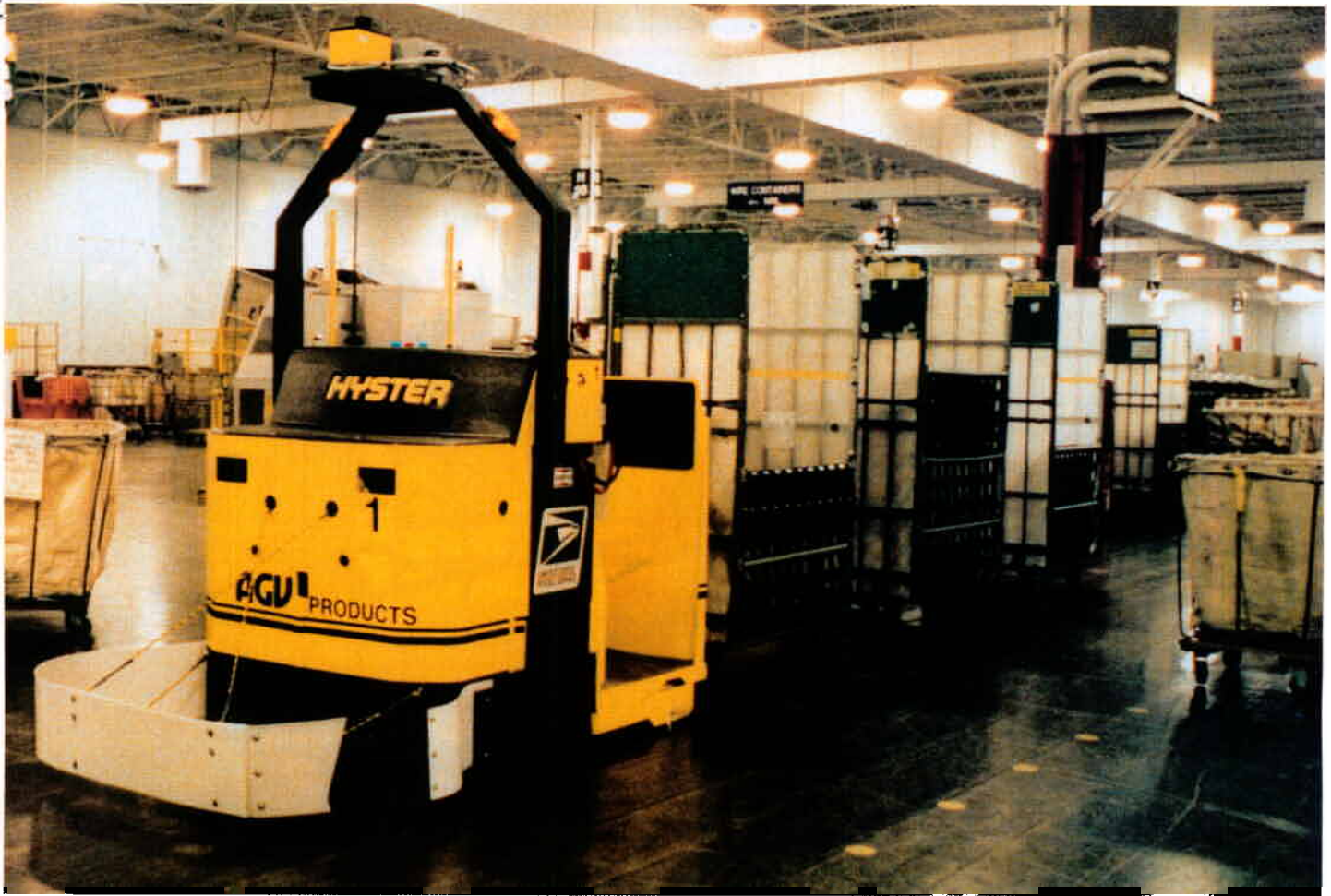
An automated towmotor pulls three general purpose containers down an aisle at the Fort Myers facility. A full GPC can weigh as much as 1,200 pounds.
