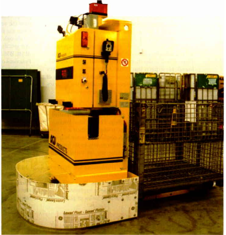
One of two automated forklifts at the Fort Myers processing operation drags an empty wire container behind it. This carrier typifies the several varieties of mail containers in the facility.
