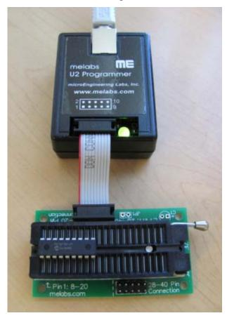
Make sure the PIC is positioned and oriented in the programmer properly before continuing.
