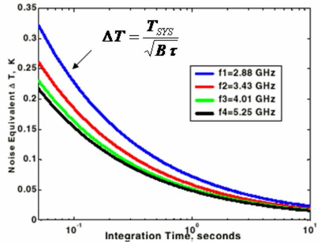
Fig. 4 Calculated sensitivity of the Miniaturized Water Vapor Radiometer (MWVR).
