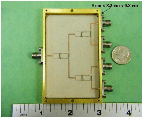
Fig. 3 Broadband Wilkinson power divider fabricated in microstrip using a high-dielectric substrate and thin-film resistors.
