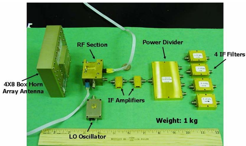
Fig. 5 Antenna and RF/IF sections of the MWVR.
