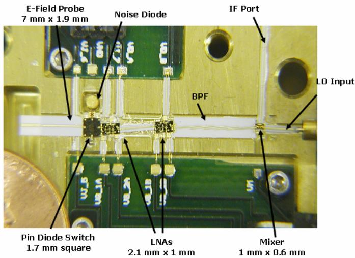
Fig. 1 RF section implemented in a multi-chip module.
