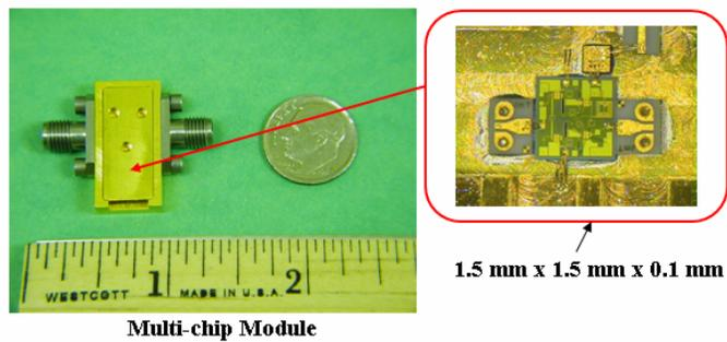
Fig. 2 Two-stage IF amplifier implemented in a multi-chip module.
