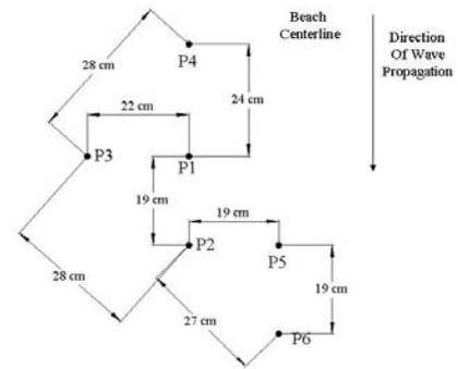
**Figure 3.** The position of the pressure transducers in the wave tank.
