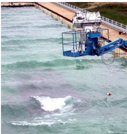
**Figure 1.** Microwave radiometers observing a breaking wave at the WindSat polarimetric frequencies (10.7, 18.7 and 37 GHz) at the OHMSETT wave basin during the POEWEX'02 experiment.
