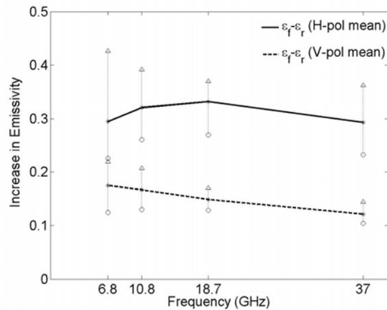
**Figure 7. Mean and azimuthal variation of increase in emissivity as a function of frequency at 53° incidence angle.**
