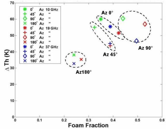
Figure 3. Measured increase in horizontal brightness temperature due to foam for three different frequencies and at four azimuth angles, all at  $53^\circ$  incidence angle.
