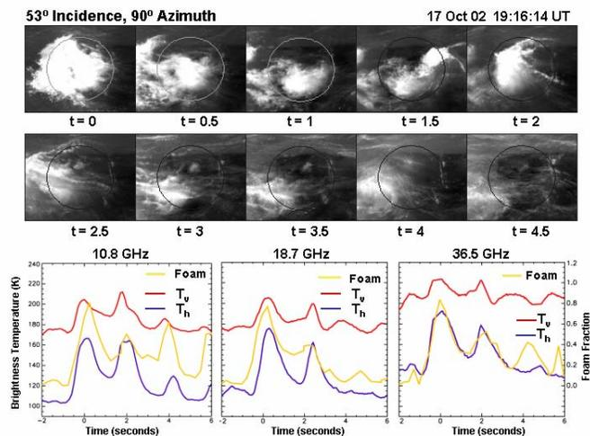
Figure 2. The top panel shows a time series of video images at a rate of 2 Hz with one of the boresighted radiometers' fields of view shown by an ellipse. The bottom panel shows the time series of vertical (red) and horizontal (blue) brightness temperatures and foam fraction in the field of view (yellow), at frequencies of 10.8, 18.7 and 37 GHz at an incidence angle of 53° and an azimuth angle of 90°. The  $t=0$  on the lower time axes corresponds to the time of the top left video image.
