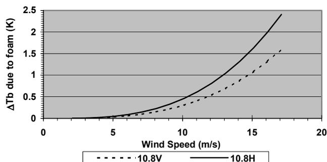
Figure 5. The increases in brightness temperatures at 10.8 GHz expected to be measured by a spaceborne radiometer, at low-to-intermediate wind speeds.
