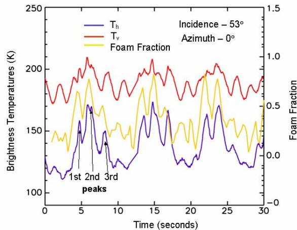
Figure 1. Radiometric brightness temperature at 19 GHz of groups of breaking waves measured at an incidence angle of 53° and azimuthal angle of 0° (looking into the direction of breaking) during POEWEX.
