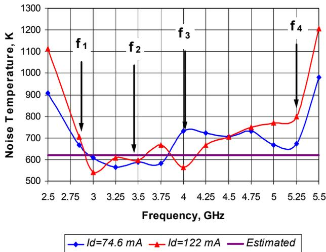
Fig. 4 Measured equivalent noise temperature of MWVR.
