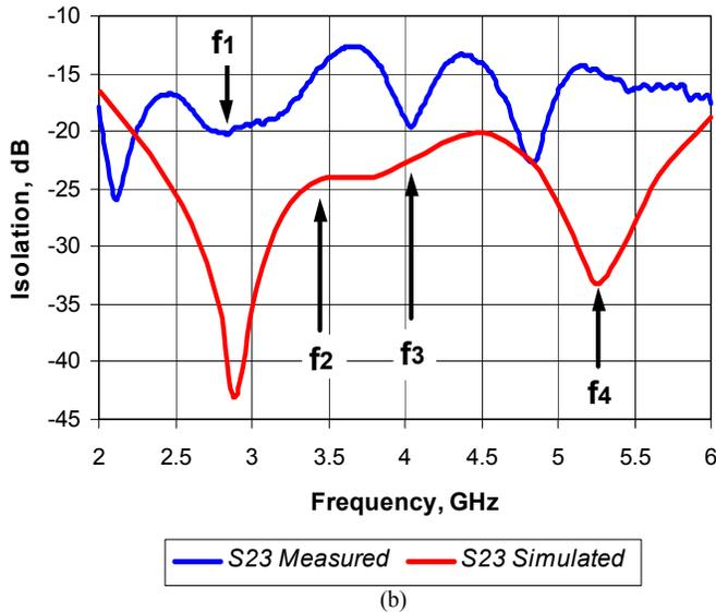
Fig. 6. Measured and simulated response of (a) input return loss and (b) isolation between two adjacent output ports of the two-section coupled microstrip power divider.
