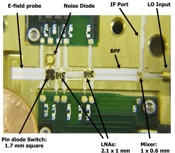
Fig. 2. RF section of MWVR.
