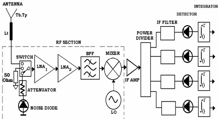
Fig. 1. Block diagram of the miniaturized water vapor profiling radiometer.
