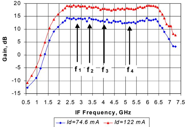
Fig. 3. Gain performance measured at IF port.
