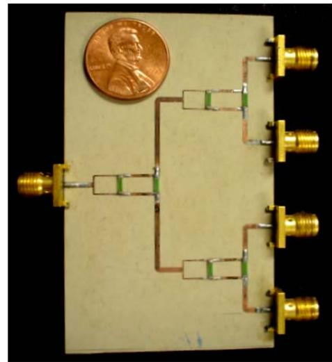
Fig. 5. Two-section coupled microstrip power divider
