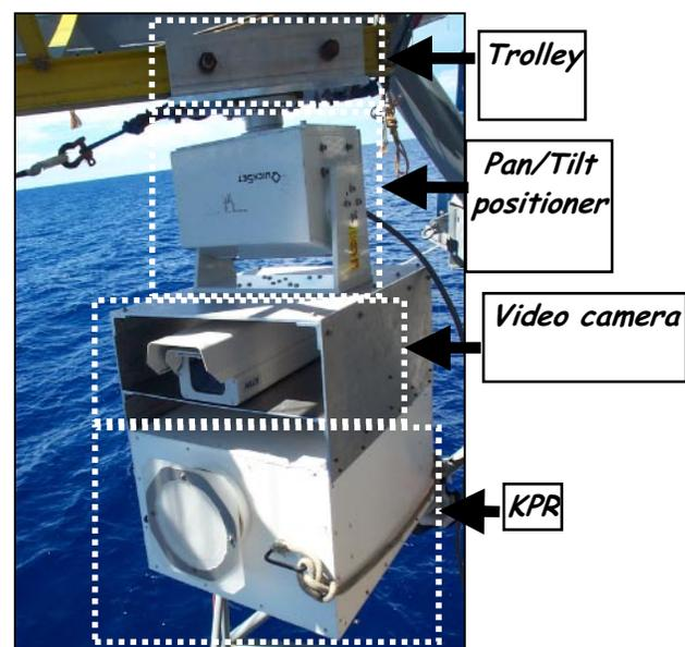
Fig. 1. KPR radiometer with a video camera and pan-tilt positioner deployed during the RED experiment. A rexolite radome was used to protect the antenna and the radio frequency components from the corrosive operational environment.
