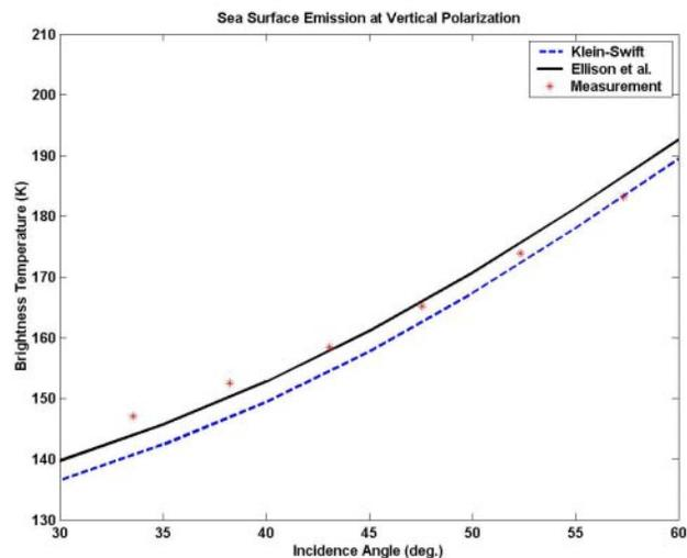
Fig. 5. Comparison at vertical polarization (Klein-Swift model--blue dashed line, Ellison model--black solid line, Measurements—red asterisks). SST = 26 °C, SSS =36 psu, WS = 8 m/s.
