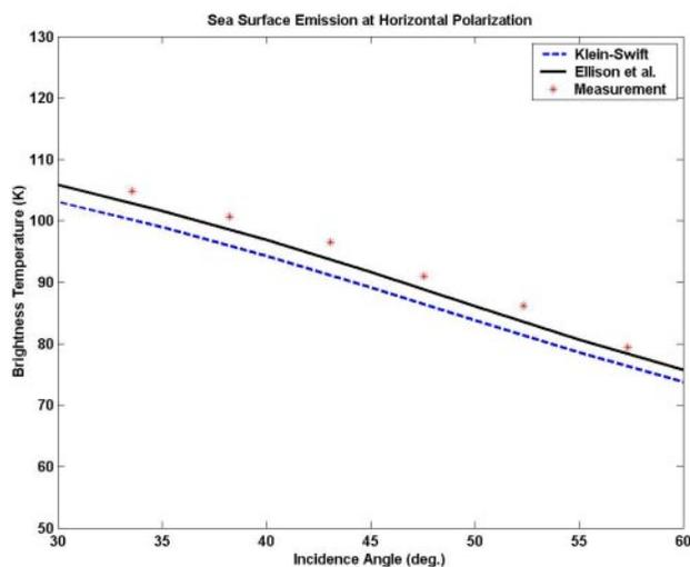
Fig. 4. Comparison of measurements and models at horizontal polarization (Klein-Swift dielectric model--blue dashed line, Ellison *et al.* model--black solid line, Measurements—red asterisks). SST = 26 °C, SSS =36 psu, WS = 8 m/s.
