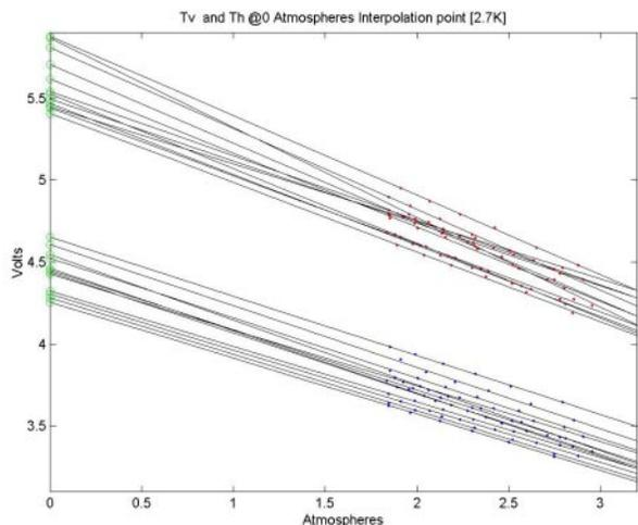
Fig. 2. Set of tip curves at both H (red dots) and V (blue dots) polarizations.
