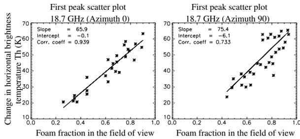
Fig. 5. Scatter plots of the change in horizontal brightness temperature versus foam fraction for azimuth angles  $0^\circ$  and  $90^\circ$ .
