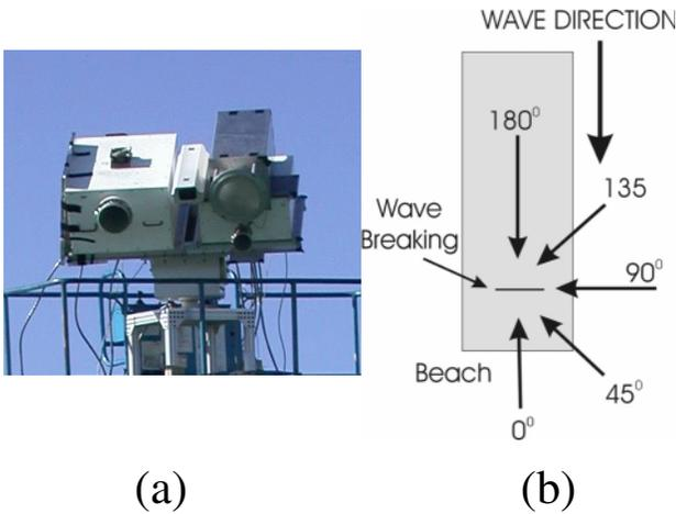
Fig. 2. (a). NRL and UMass polarimetric radiometers with a boresighted video camera in the basket of a boom lift crane. (b). The five azimuthal positions of the radiometer.
