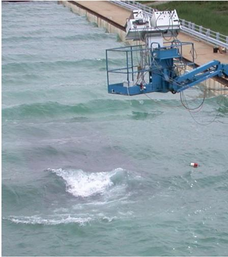
Fig. 1. Radiometers observing a breaking wave at the Ohmsett facility during POEWEX.
