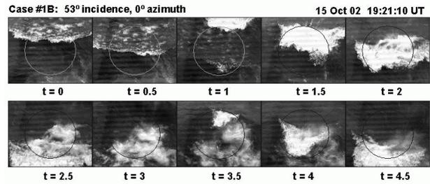
Fig. 3. A time series of video images (every half-second) of several breaking waves measured by a bore sighted video camera for azimuth angle of  $0^\circ$  and incidence angle of  $53^\circ$ .
