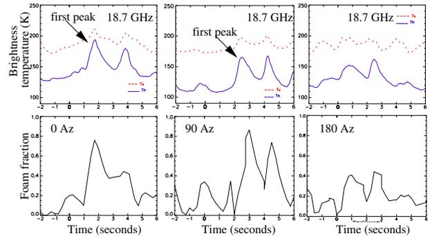
Fig. 4. The top row consists of time series of radiometric brightness temperatures,  $T_v$  and  $T_h$  shown as dotted and solid lines, respectively, for azimuth angles  $0^\circ$ ,  $90^\circ$  and  $180^\circ$ , from left to right. The bottom row consists of foam coverage time series recorded simultaneously. The plots on the left correspond to the video images shown in Fig. 3.
