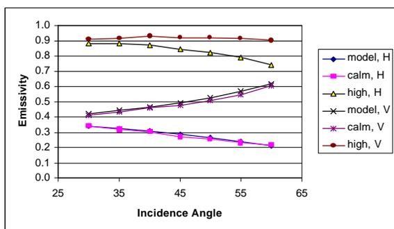
Fig. 4. High-level foam and calm water emissivity at 10.8 GHz, horizontal and vertical polarization. NRL model for calm sea water also shown.
