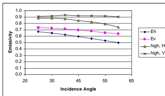
Fig. 7.  $E_h$  and  $E_v$  are model plots from Stogryn [3]. High H and High V are the 10.8 GHz H and V emissivity plots taken from Fig. 4.
