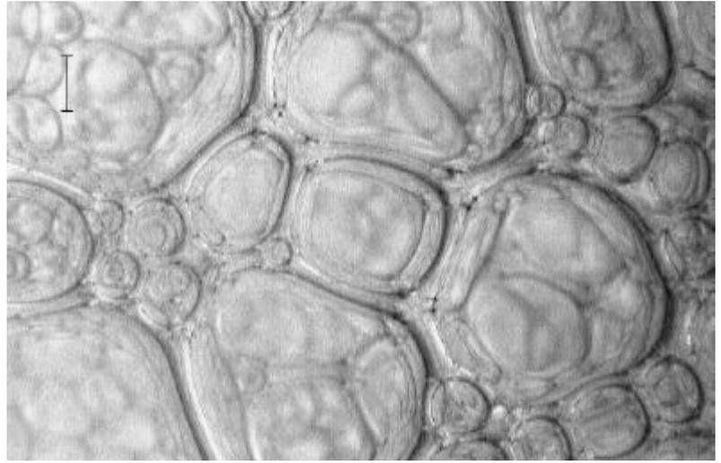
Fig. 2. Typical image of the bubble microstructure in the foam interior as recorded by an underwater camera mounted near the center of the foam raft. The scale bar shown in the upper left corner represents a distance of 500 micrometers.
