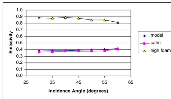
Fig. 6. High-level foam and calm water emissivity at 10.8 GHz for left circular polarization.
