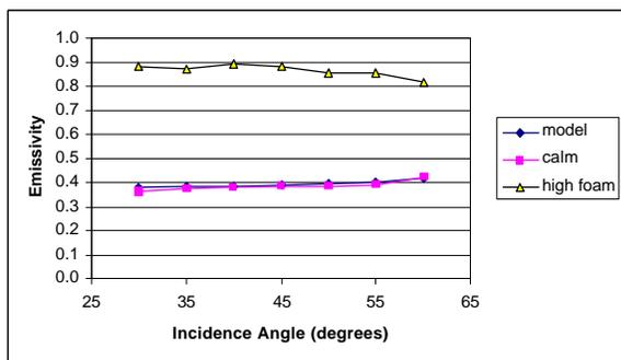
Fig. 5. High-level foam and calm water emissivity at 10.8 GHz for -45 degree linear polarization.
