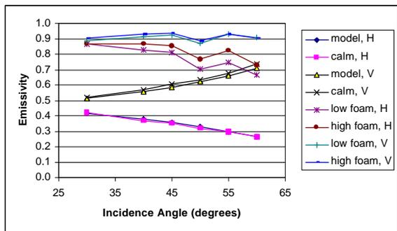
Fig. 3. Emissivity results at 36.5 GHz. Horizontal and vertical polarization, high and low foam. NRL model values for calm water are shown with the experimental measurements.
