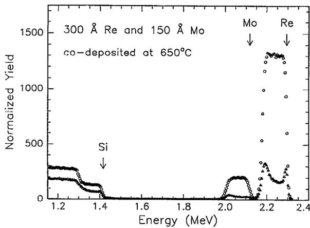
FIG. 3. 2.5 MeV  $^4\text{He}$  backscattering spectra of  $\text{Re}_x\text{Mo}_{1-x}$  deposited onto  $\text{Si}(100)$  at  $650^\circ\text{C}$  for  $x=0.68$ : (O) random beam incidence ( $7^\circ$  off sample normal) and ( $\Delta$ ) channeled in the  $\text{Si}(100)$  direction. The scattering angle of the detected particles is  $170^\circ$ .
