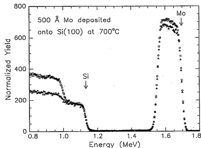
FIG. 1. 2.0 MeV <sup>4</sup>He backscattering spectra of 500 Å of Mo deposited on  $\text{Si}(100)$  at 700 °C: (O) random beam incidence (7° off sample normal) and (Δ) channeled in the  $\text{Si}(100)$  direction. The scattering angle of the detected particles is 170°.
