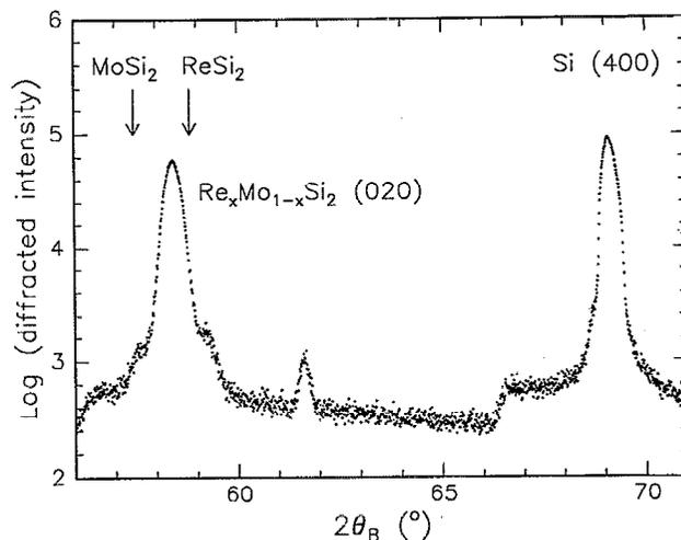
FIG. 2. X-ray  $\theta$ - $2\theta$  diffraction of  $\text{Re}_x\text{Mo}_{1-x}$  deposited onto  $\text{Si}(100)$  at 650 °C for  $x=0.82$ . The arrows indicate the  $2\theta$  values for the two binary silicides. The peak at  $2\theta \approx 61.5^\circ$  and the absorption edge at  $2\theta \approx 66.5^\circ$  are artifacts caused by a Ni filter used in the experiment.
