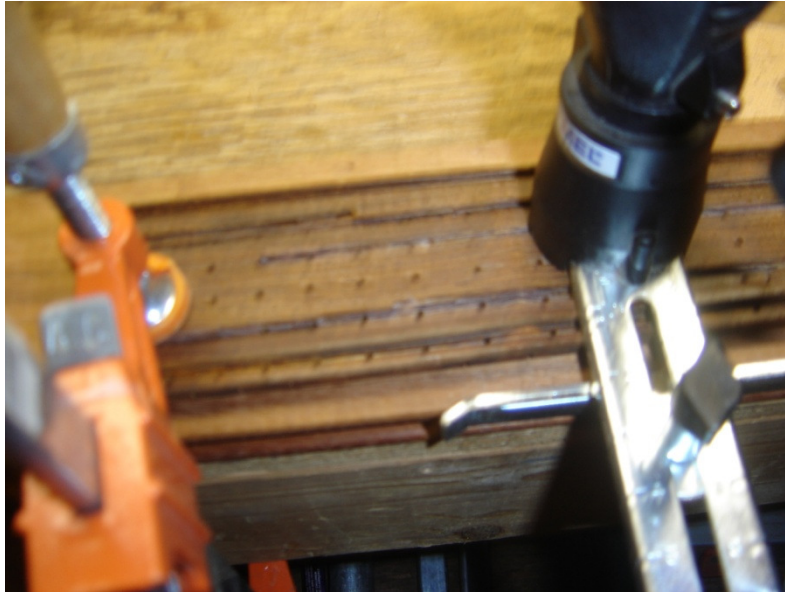
Figure 6 – Dremel Routing Jig
