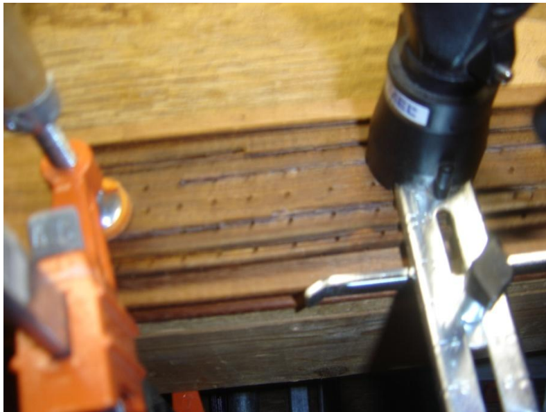
Figure 6 - Dremel routing jig
