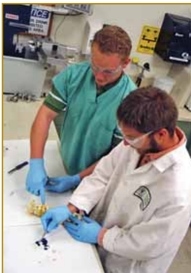
CSU junior mechanical engineering and biomedical science double major, Dan Woldtvedt (above left), collaborated with doctoral student Wes Womack (right) to create a three-dimensional model of the cartilage in the human spinal cord. Creating the model involved dissecting cervical vertebrae, sectioning them into 1 millimeter slices, and photographing each slice. Womack wrote a mathematical code to define the cartilaginous regions on each slice in three-dimensional coordinates. Their work won Woldtvedt the 2007 Biomedical Engineering Society Undergraduate Research and Design Award.
