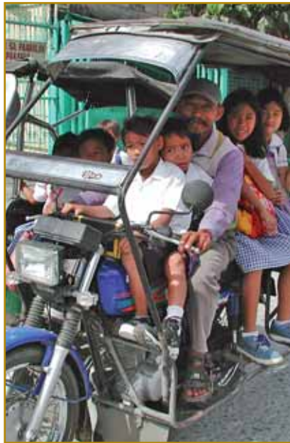
A retrofit kit initially designed as a senior design project to reduce the emissions of snowmobiles is being applied to two-stroke motorcycle taxis (motorcycle school bus shown above) in Third World countries. Envirofit, an independent nonprofit company started at Colorado State in 2003, works to create and disseminate direct injection retrofit kits to reduce fuel and oil consumption by 35–50 percent and cut emissions by as much as 90 percent.
