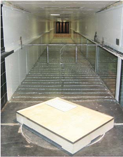
Fig. 2. Representative Wind Tunnel Configuration for Testing of Models of Photovoltaic Roofing Systems, at Wind Engineering and Fluids Laboratory, Colorado State University
