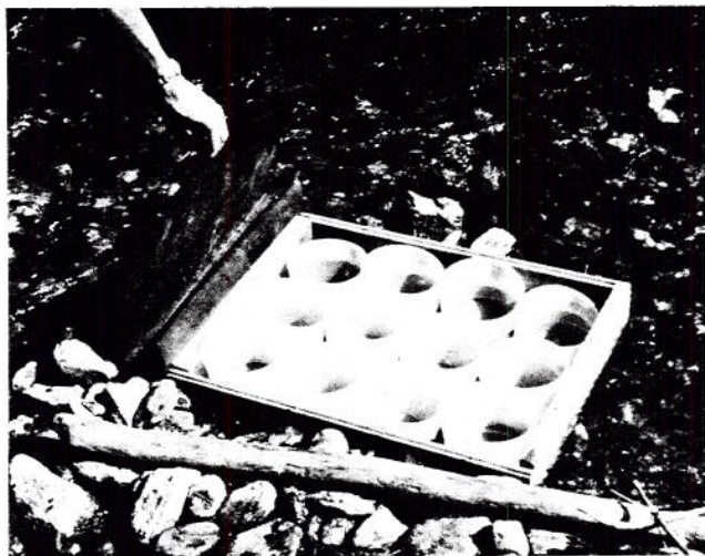
Figure 5. The arrangement used in the insolation study. The black felt paper provided shade for six of the containers, while the others remained exposed to sunlight.
