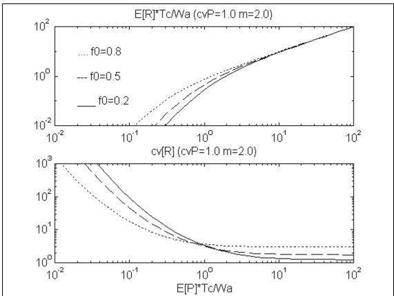
Fig. 3 - Expected non-dimensional runoff and its coefficient of variation as a function of the non-dimensional precipitation intensity
