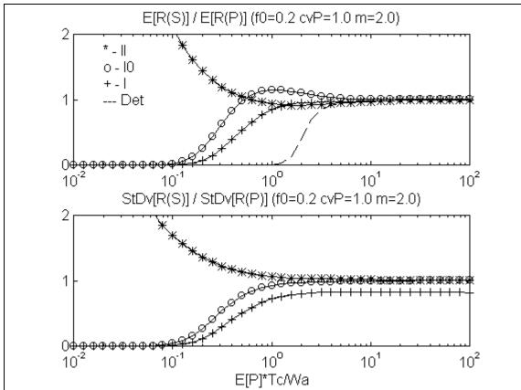
Fig. 4 - Ratios between the means and the standard deviations of the QPF-based and the "true" surface runoff, R(S) and R(P), for various probabilistic parametrization of the forecasted precipitation S, assuming a zero-rainfall probability f0=0.2.
