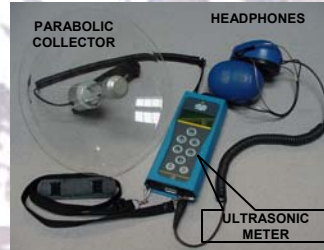
Fig. 4. SDT170 air leak detector used to troubleshoot, converted ultrasound to audible signals for synchronizing communications.
