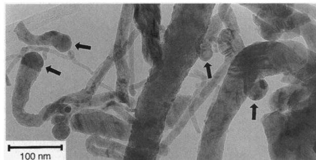
**Fig. 4.** A TEM image of polycrystalline InP fibers obtained from reaction 1a (PhSH catalyst, refluxing toluene solution). The arrows point to the In flux particles (frozen droplets) at the fiber tips.
