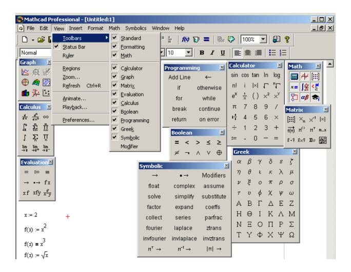
The MathCAD workspace is considerably different from most "spreadsheet style" data analysis program (like excel). Equations, data tables, graphs and descriptive text can all be combined in one MathCAD document, making this software particularly handy for application
