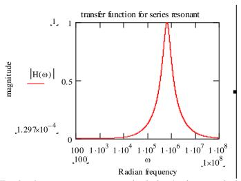
To checks or compare your calculation/estimate solution of RLC series resonant inverter circuit. You can use the Pspice software tool to run simulation of your circuit. This can done by simply design a RLC series resonant inverter circuit on the Pspice schematic, save and run simulation of the circuit. The Pspice will give you a graph of the transfer function of your circuit. Figure below is the Pspice result of RLC series resonant inverter circuit.
