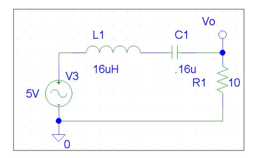
To Plots the transfer function of this circuit in MathCAD software, here is how you do it
