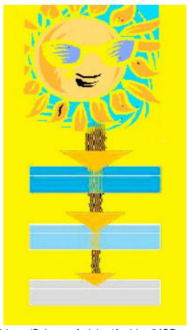
A one-layer solar cell is limited to 20 percent efficiency in converting light to power, but materials with different bandgaps can be stacked in multijunction cells. Each layer responds to a different photon energy of sunlight to achieve 40 % efficiency.
