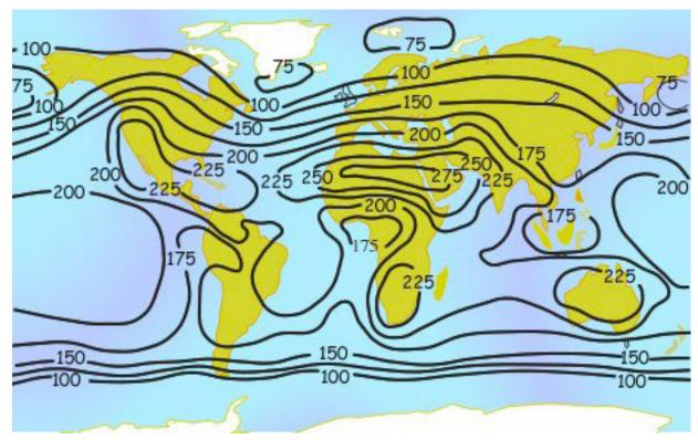
24 hour/365 day mean solar radiation received at the surface, in W/m2. It oscillates between a maximum of 275 M/m $^2$  in the deserts of the Middle East, to a low of 75 W/m $^2$  for misty isles in the Arctic.
