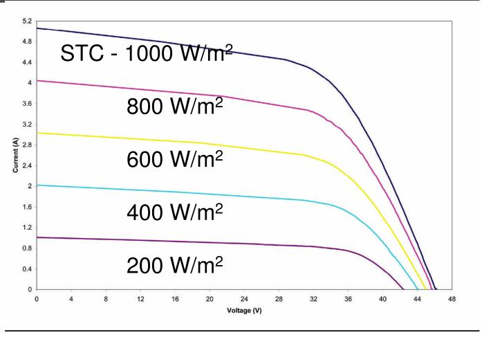
Air Mass 1.5 and 25C cell temperature
