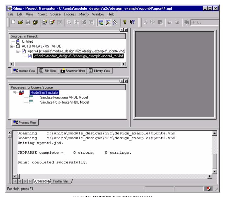
Figure 14: ModelSim Simulator Processes
