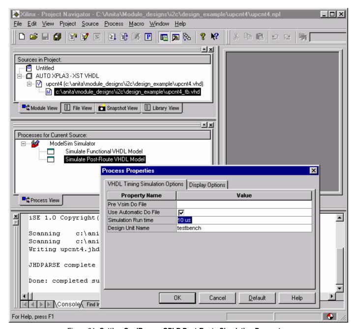
Figure 24: Setting CoolRunner CPLD Post-Route Simulation Parameters
