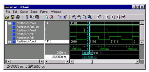
Figure 25: CoolRunner CPLD Post-Route Simulation Results
