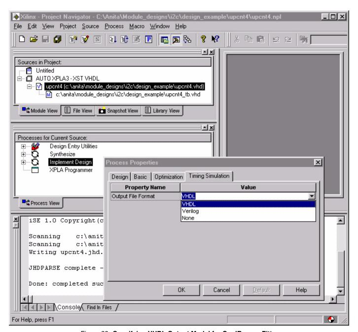
Figure 23: Specifying VHDL Output Model for CoolRunner Fitter
