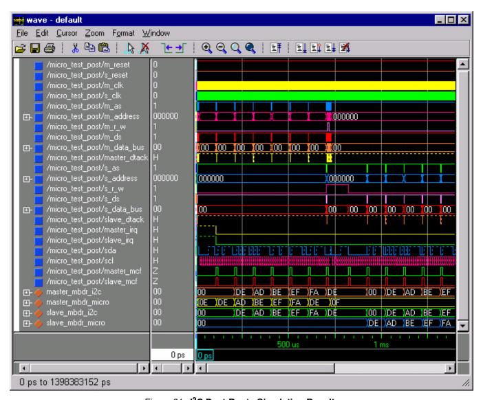
Figure 31: I<sup>2</sup>C Post-Route Simulation Results
