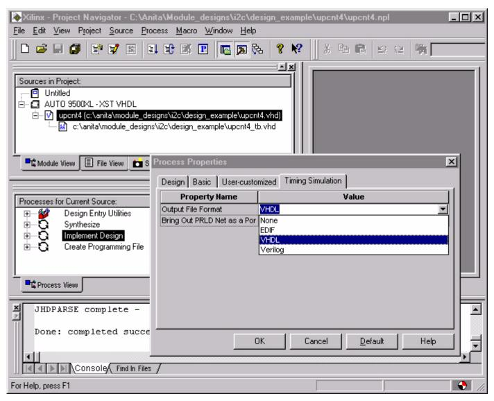
Figure 19: Specifying VHDL Output Model for XC9500 Fitter
