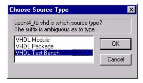
Figure 13: Specifying UPCNT4\_TB.VHD as VHDL TestBench
