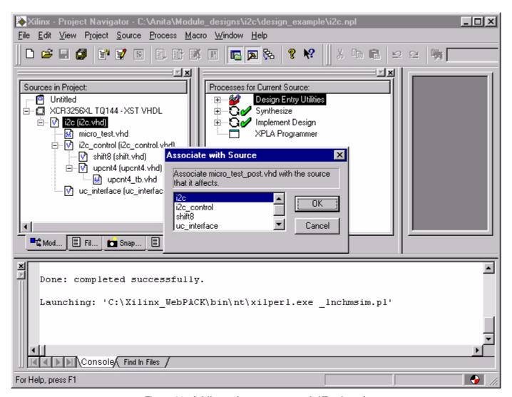
Figure 29: Adding micro\_test\_post.vhd Testbench
