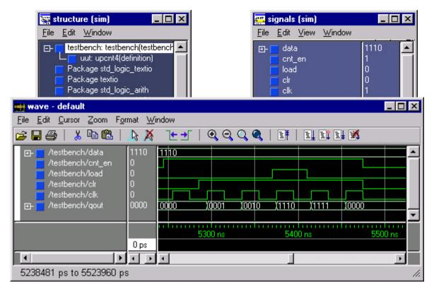
Figure 17: ModelSim Structure, Signal, and Wave Windows
