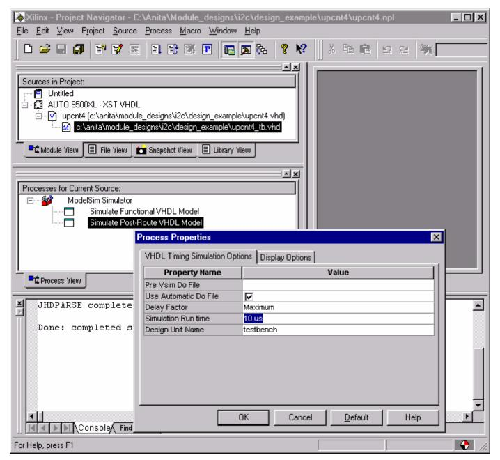
Figure 20: Setting Post-Route Simulation Parameters
