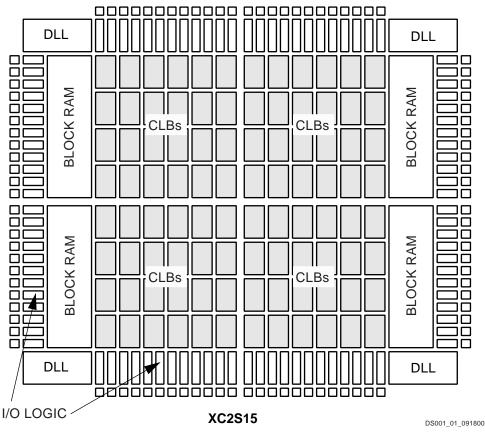
Figure 1: Basic Spartan-II Family FPGA Block Diagram
