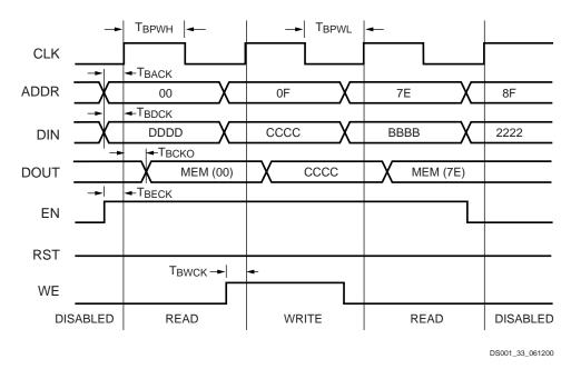
Figure 32: Timing Diagram for Single-Port Block RAM Memory
