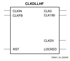
Figure 23: High-Frequency DLL Symbol CLKDLLHF
