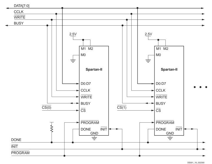
Figure 17: Slave Parallel Configuration Circuit Diagram
