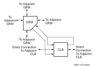
Figure 5: Spartan-II Local Routing
