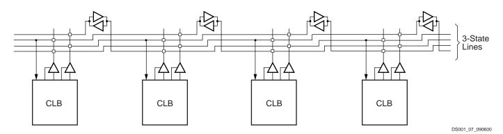
Figure 6: BUFT Connections to Dedicated Horizontal Bus Lines
