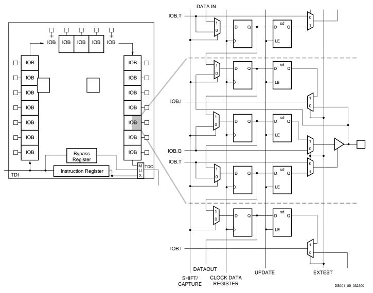
Figure 8: Spartan-II Family Boundary Scan Logic
