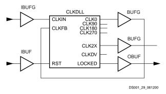
Figure 28: DLL Deskew of Clock and 2x Multiple
