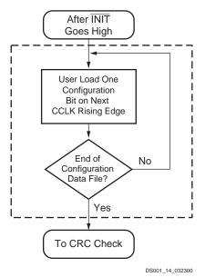
Figure 13: Loading Serial Mode Configuration Data
