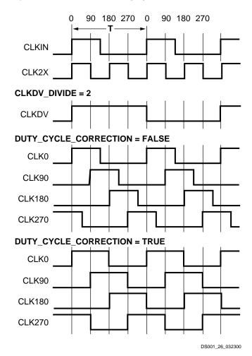
Figure 25: DLL Output Characteristics
