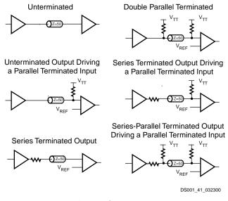
Figure 40: Overview of Standard Input and Output Termination Methods
