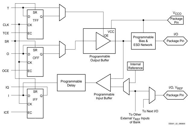
Figure 1: Spartan-II Input/Output Block (IOB)
