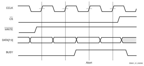
Figure 20: Slave Parallel Write Abort Waveforms
