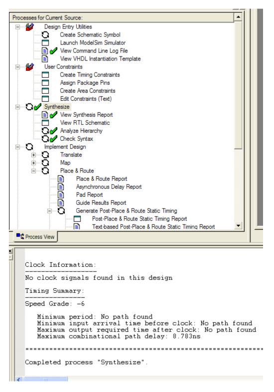
7. Now you are ready to route, place and map your netlist onto a Spartan II FPGA (which is used on the XESS XSA-50 FPGA protoboard). To route, place and map your design, double left click on "Implement Design" in the "Processes for Current Source:" window or right click on "Implement Design" and select "Run" or "Rerun" (the latter instructions will depend on whether or not you have selected to route, place and map your design on an earlier occasion). The following will result:
