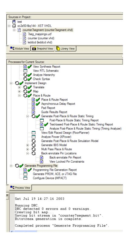
10. Now you are ready to download your bit stream onto the XESS XSA-50 FPGA protoboard. To accomplish this, we must use the XESS GXSLOAD utility. The utility can be found in
