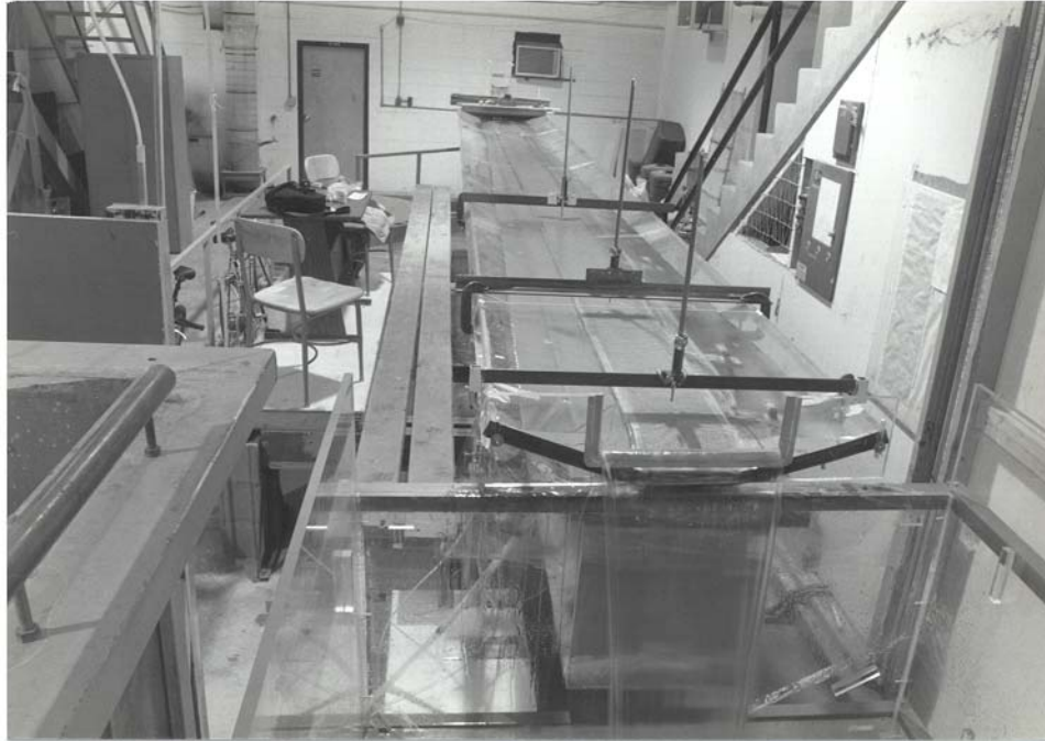
Figure 3.1: Three Point Gages used to Measure Water Depth.
