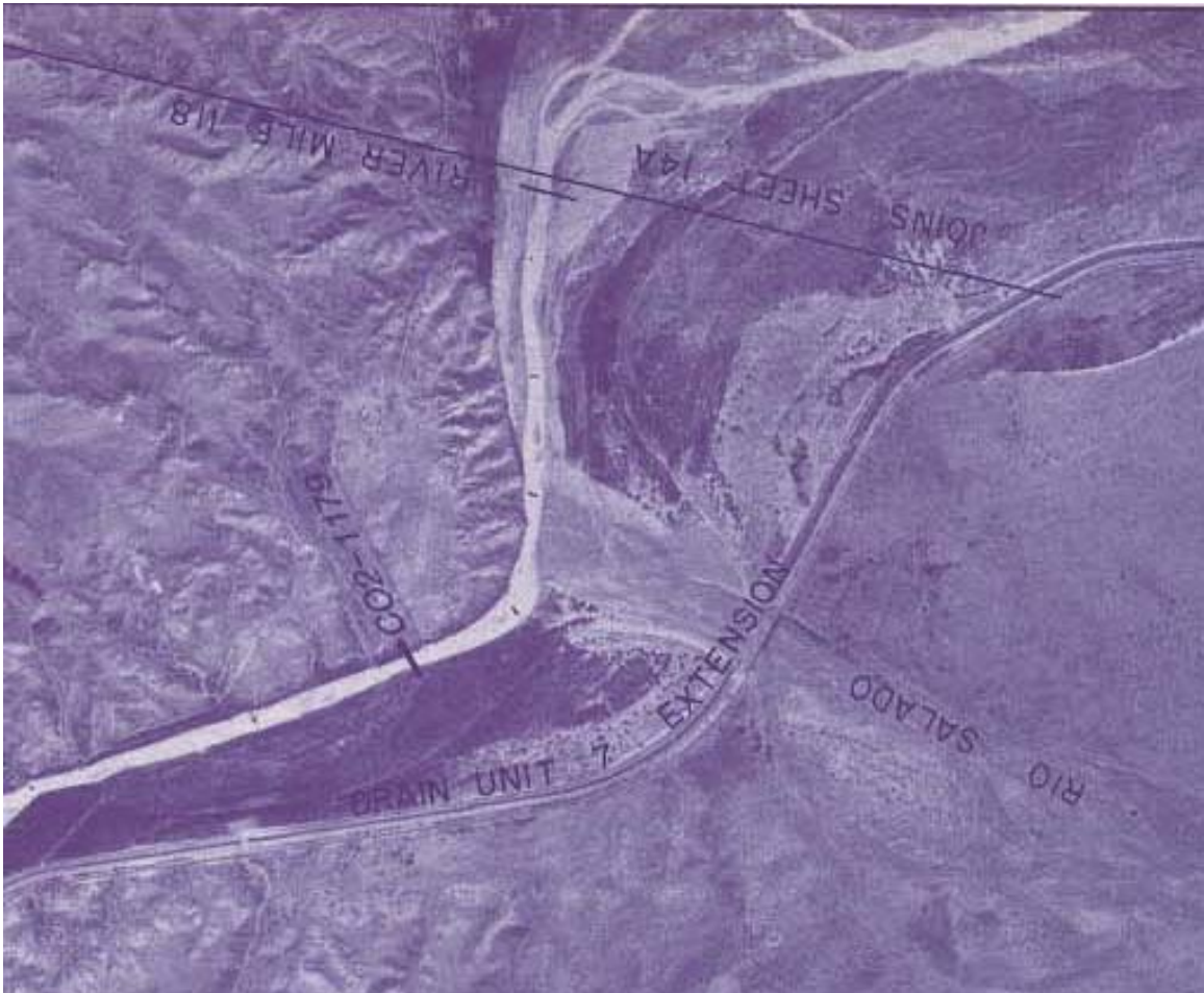
Figure 4.1. Rio Grande flowing from left to right. Notice the abrupt change of course as the Rio Grande reaches the delta of the Rio Salado. The channel also narrows considerable at the confluence. Several abandoned channels or terraces are evident in the photo to the right of the current channel location. The Arroyo Rosa de Castillo enters the Rio Grande near the top center in the photo.
